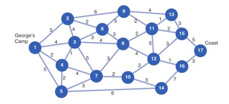
Determine the shortest (time) path for George to take and indicate the total time. Assume that all edges can be travelled in both directions; you may use either Excel or the Dijkstra algorithm.
