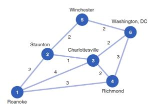
The time, in hours, between cities (which is affected by the type of road and the number of intermediate towns) is shown along each branch. Determine the shortest route that the Millstone family can travel from Roanoke to Washington, DC. Assume that the family will only travel in a north-east direction, that is, assume edges are directed from lower node index to larger node index. Use the Dijkstra algorithm by hand.
